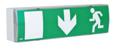
In its traditional form it is the cheapest light. Recommended mainly to be mounted on sidewalls. It has a smaller size pictogram, thus it is an exit showing light with a higher light emission that is primarily recommended to be used in small rooms, turns and above doors. Its IP42 protection makes applicable to industrial buildings, and engineering rooms.
